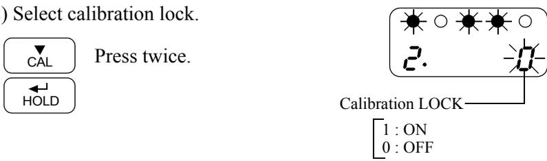
Use **GAIN** and **CAL** key to set the calibration lock of ON (1). then use **HOLD** key to validate the setting.
