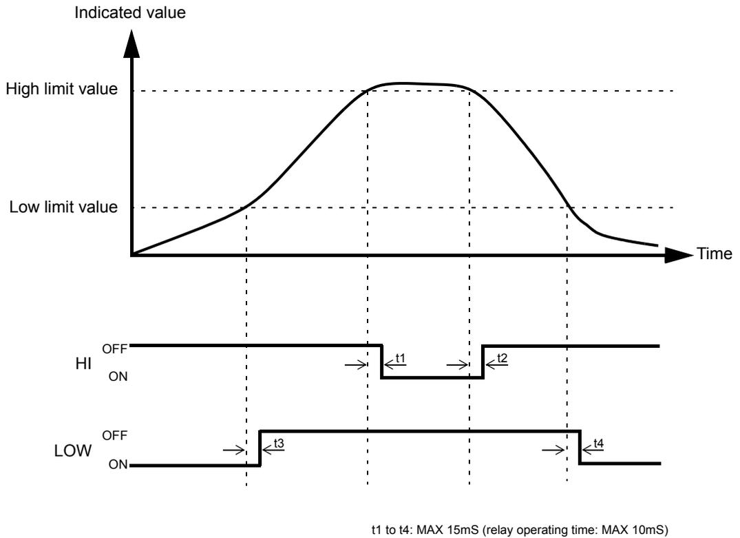
t1 : Time from when the indicated value exceeds the high limit set value to when the relay turns ON
