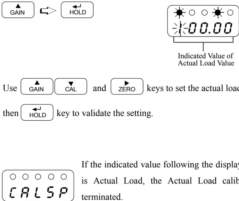
Use **GAIN**, **CAL**, and **ZERO** keys to set the actual load value, then **HOLD** key to validate the setting.
