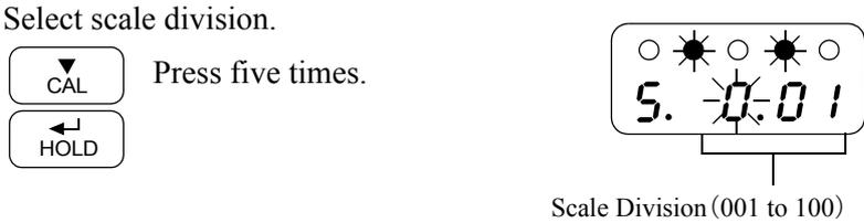
Use **GAIN**, **CAL** and **ZERO** key to set the scale division, then use **HOLD** key to validate the setting.
