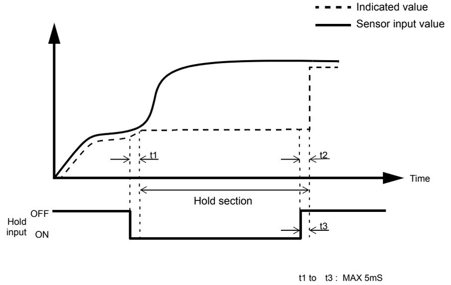
t1 : Time from when the hold signal is inputted to when the indicated value is held
