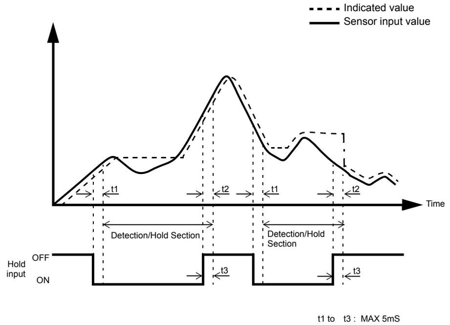
$t_1$  : Time from when the hold signal is inputted to when the indicated value is held
