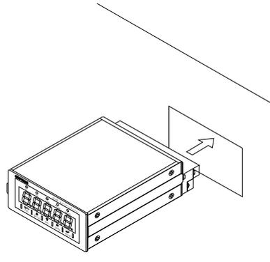
4. Mount the guide rails from the back, and fix them with the attached screws.
