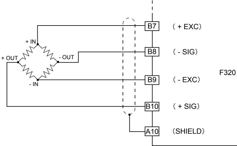
◇ 6-wire Strain Gauge Sensor
